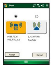
**Connections:** Configuration of the transmission of RTK corrections via radio and internet
